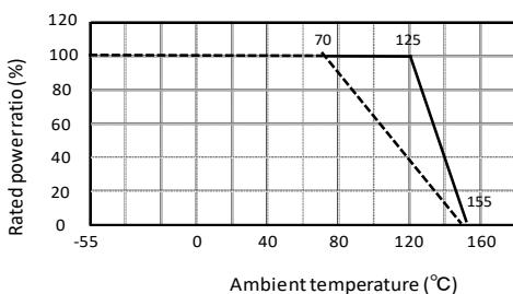
\* Rated power of the resistor is the maximum power
