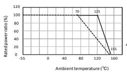
\*Rated power of the resistor is the maximum power which can be loaded continuously at the ambient temperature of 70°C. For the ambient temperature above 70, please use the item according to the load derating curve (dotted line)
