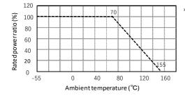
\* Rated power of the resistor is the maximum power which can be loaded continuously at the ambient temperature of 70 °C. For the ambient temperature above 70°C, please use according to the load derating curve (dotted line). Please note that the component surface temperature does not exceed operating temperature range.
